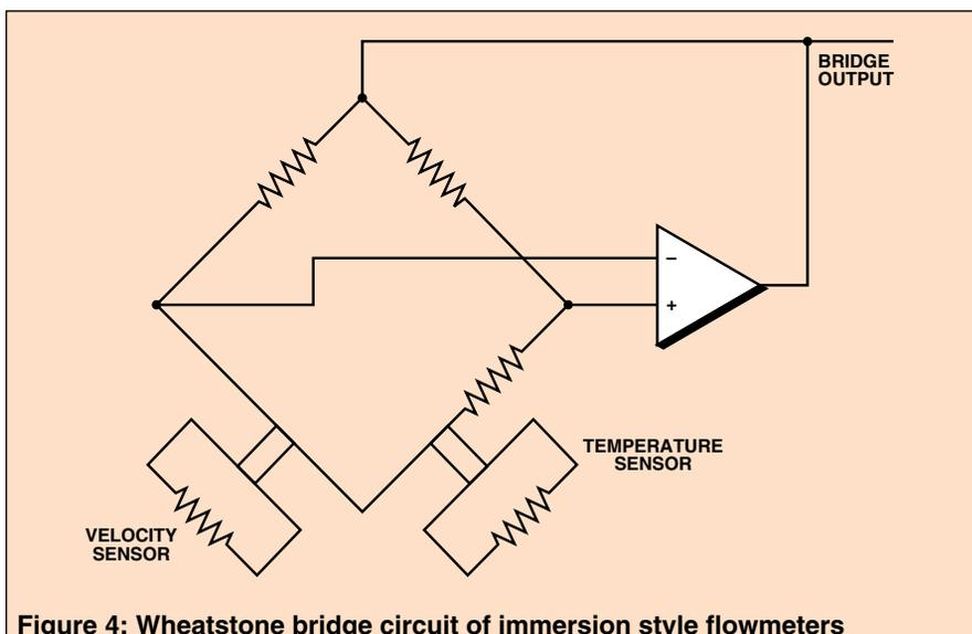
Figure 4: Wheatstone bridge circuit of immersion style flowmeters
