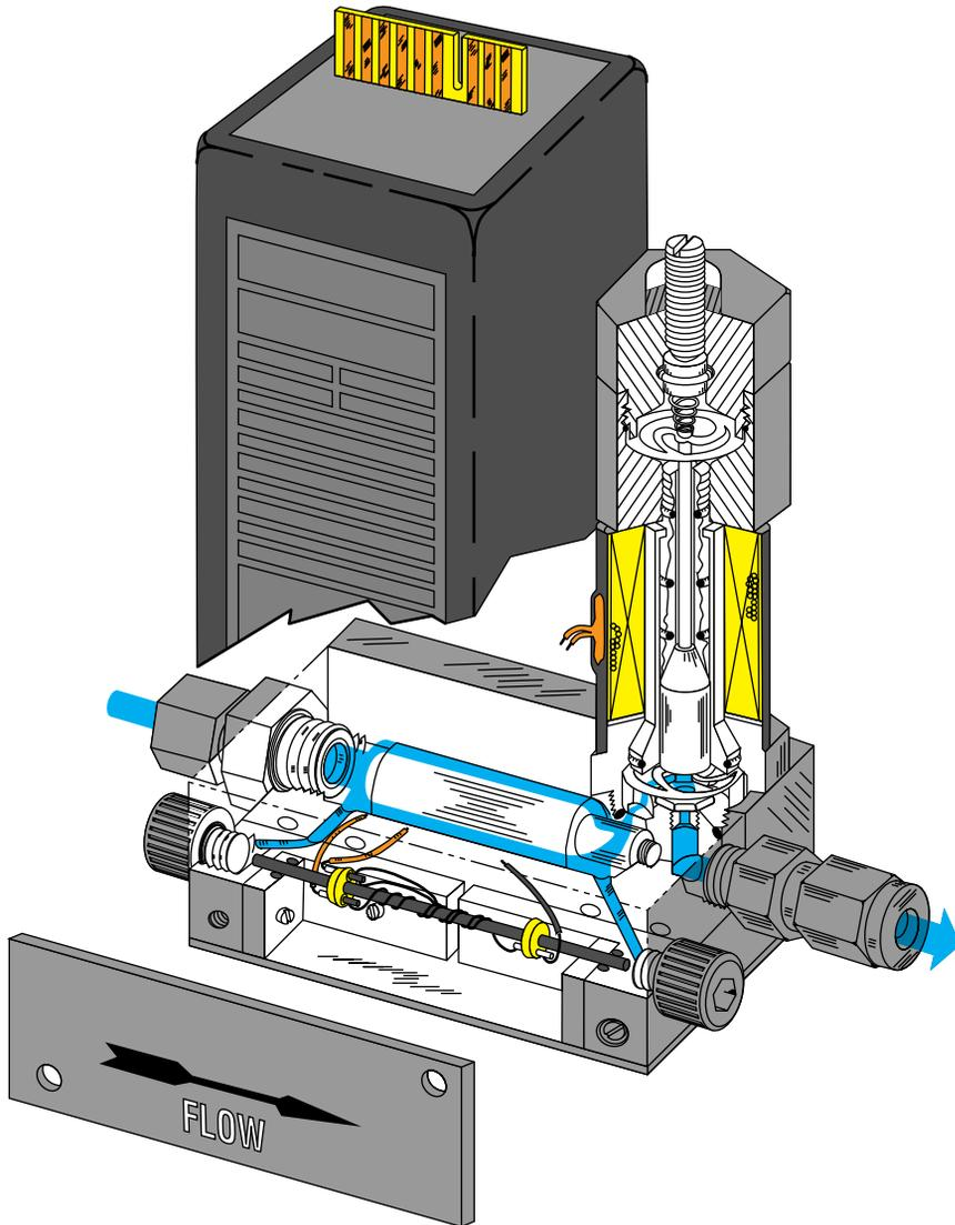
Figure 3: Heated tube mass flow controller
