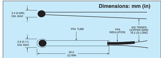
some protection from humidity and or corrosion. It is the epoxy bead-type thermistor that is used in Omega's thermistor temperature sensor products.
