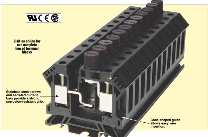
OMEGA's OMTBV7-W terminals are designed to meet the three most important criteria when selecting a terminal block line – ease of wiring, secure connections and durability. The line is also comprehensive, offering a wide array of terminal types for most circuits and functions, from control to low level power.
