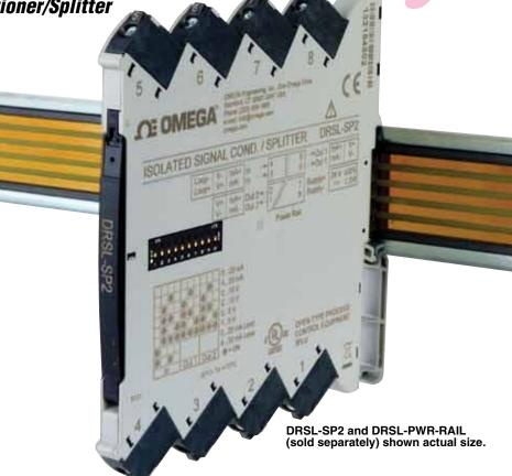
The DRSL-SP2 isolated signal conditioner/splitter provides a competitive choice in terms of both price and technology for galvanic isolation of process voltage or current signals to SCADA systems or PLC equipment. Two process outputs are provided which mirror the single process input.
