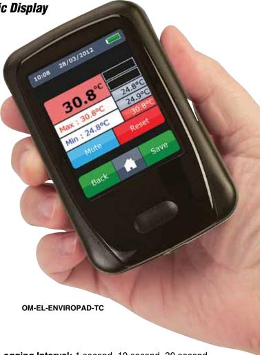
**Logging Interval:** 1 second, 10 second, 30 second, 1 minute, 5 minute, 30 minute, 1 hour, 6 hour, 12 hour
