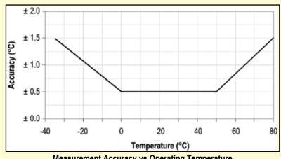
**Measurement Accuracy vs Operating Temperature**
