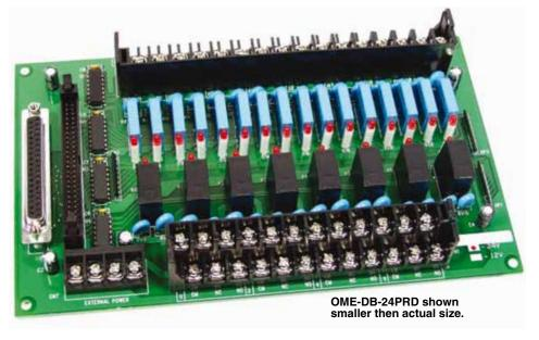
**Maximum Switching Voltage:** 270 Vac, 150 Vdc
