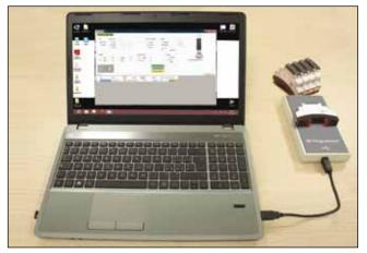
TX400-RFID programmer shown connected to PC.
