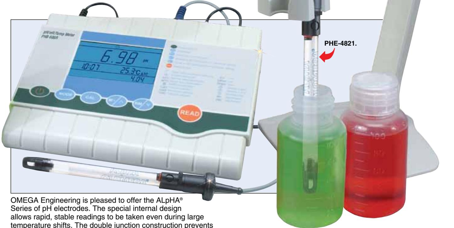
OMEGA Engineering is pleased to offer the ALpHA® Series of pH electrodes. The special internal design allows rapid, stable readings to be taken even during large temperature shifts. The double junction construction prevents silver ions from contacting the sample, eliminating reactions with heavy metals, sulfides, and proteins. ALpHA Series electrodes are available in a variety of styles to suit a wide range of applications.
