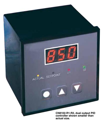
ovens and packaging machinery. As a high-limit device, these controllers have a normally energized SPST latching output relay which becomes de-energized whenever the process variable (PV) exceeds a selected setpoint value. Reset of the latching output relay is done by holding the parameter button for 3 seconds on the front panel of the controller, or by cycling power to the controller.
