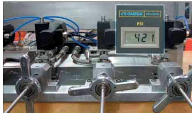
Probes are subjected to a leak test at the welded thermocouple junction (hot end) with a pressurization greater than 2.5 MPa (362 psi).
