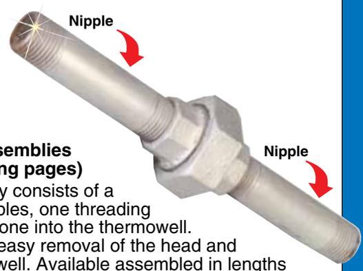
A Type 4 assembly consists of a union and two nipples, one threading into the head and one into the thermowell. This type permits easy removal of the head and element from the well. Available assembled in lengths between 76 mm (3") and 305 mm (12").
