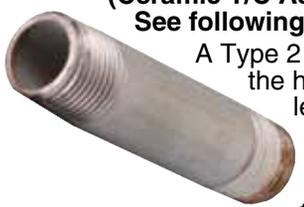
A Type 2 assembly is used to connect the head to a thermowell. The length is measured from the bottom of the head to the top of the well. Available assembled in lengths of 0", 13 mm (1/2"), 25.4 mm (1"), 38 mm (1 1/2"), 51 mm (2"), 64 mm (2 1/2"), 76 mm (3"), 102 mm (4"), and 127 mm (5").
