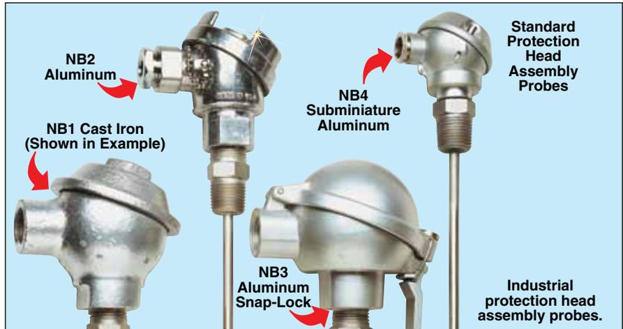
The 1/2 NPT mounting thread allows 1/4" OD industrial protection head assemblies to be put directly into OMEGA® thermowells whose bore is 0.260" without having to use any additional hardware. In this case, the probe length must be the same as the element (stem) length of the desired thermowell.
