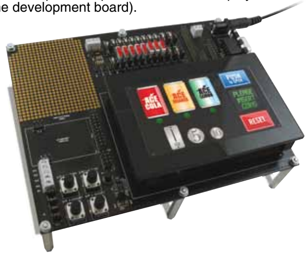
OM-SGD-43-A display shown connected to development board. Shown smaller than actual size.
