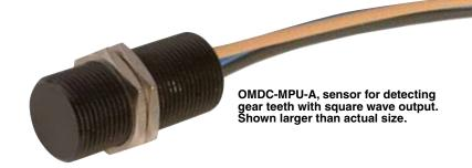
Installation and Wiring: The OMDC-MPU-A Series must be installed so that the mounting axis is perpendicular to the direction of rotation. The flat side of the sensor housing must be parallel to the direction of the gear rotation.
