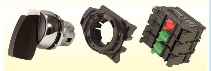
OMPBD7M-HM22PX01, two way metal selector switch with long knob. Each unit includes tool-less mounting latch and one normally closed contact block. Shown with two additional (up to 6 total per operator possible) normally open contact blocks, model OMPBD7-X10.
