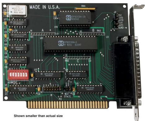
The CIO-DIO24/CTR3 combines digital input/output and counters on one board. It has the digital lines common to the PIO-12, PIO-24 and CIO-DIO24 boards, and is also connector compatible with them.
