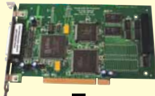
iNET-200 , instruNET controller card with PC interface for Windows based PCs.
