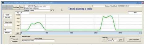
Windows software showing weight of truck passing a scale.
