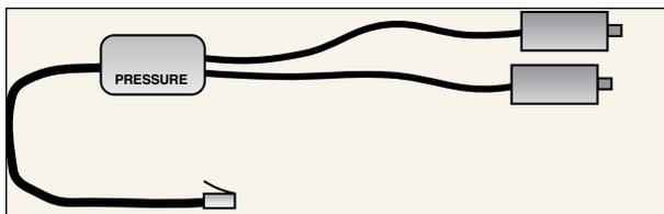
**Adaptor Type:** Complete with two pressure sensors and connecting cable to logger
