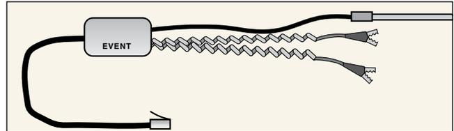
**Adaptor Type:** Complete with precision temperature sensor and event probe and connecting cable to logger
