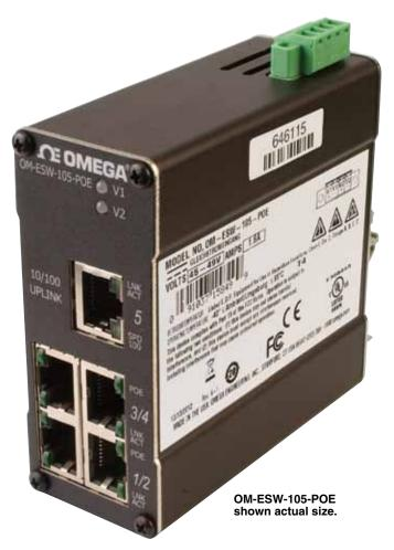
The OM-ESW-105-POE also supports up to 2000 MAC addresses, enabling these products to support extremely sophisticated and complex network architectures.
