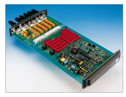
**DIGITAL CHANNELS 19 & 20 Isolation Between Channels:**500 V
