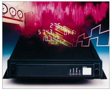
16-bit analog measurement with digital input detection – status, time, frequency, counts – and the facility for external digital output make the OM-IMP-3595 a cost-effective and flexible solution to many data acquisition applications.
