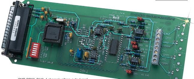
OMB-DBK2, \$649, 4-channel voltage-output card, shown smaller than acutal size
