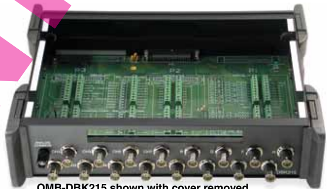
OMB-DBK215 shown with cover removed, providing access to all screw terminals, shown smaller than actual size
