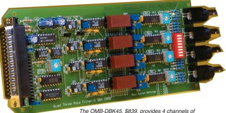
The OMB-DBK45, \$839, provides 4 channels of simultaneous sample and hold, as well as low-pass filtering
