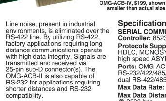
Balanced differential drivers and receivers are utilized to provide RS-422 and RS-485 communications. Selectable interrupts (IRQ levels) increases the card's versatility. Distances of 5000 ft in noisy industrial environments aré easily accommodated with the OMG-ACB.
