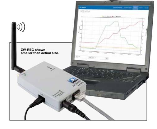
The ZW-REC offers expanded functionality over previous wireless receivers. The ZW-REC can connect to up to 128† sensors at once. The built-in web server supports encryption to protect your sensitive data. Email alarms can be sent using OMEGA Dashboard.
