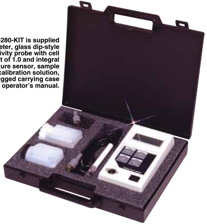
The CDH-280 conductivity meter is a basic, simple-to-operate instrument with four user-selectable ranges. It features automatic temperature compensation, a fixed 2%/°C temperature coefficient and a rugged splashproof enclosure.
