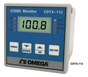
Weight CDTX-111: 580 g (20.4 oz) CDTX-112: 650 g (22.9 oz) Dimensions CDTX-111: 96 × 48 × 110 mm (3.78 x 1.89 x 4.33") **CDTX-112:** 96 × 96 × 110 mm (3.78 x 3.78 x 4.33") Mount Type: Panel Cut-Out Size CDTX-111: 92 × 44 mm (3.6 x 1.73") **CDTX-112:** 92 × 92 mm (3.6 x 3.6") Enclosure Rating: IP54 Environmental Operating Ambient Temperature: -10 to 55°C (14 to 131°F) Requirements Relative Humidity: 5 to 95% non-condensing Maximum Operating Altitude: 3000 m (10,000')
