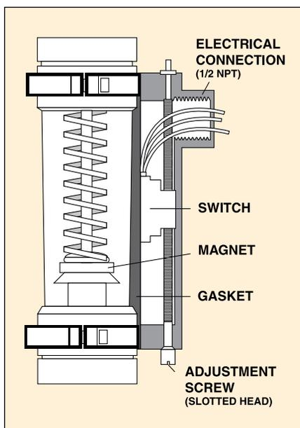
Note: Switch activates over a 25% of full scale band; above and below this band, the relay deactivates.
