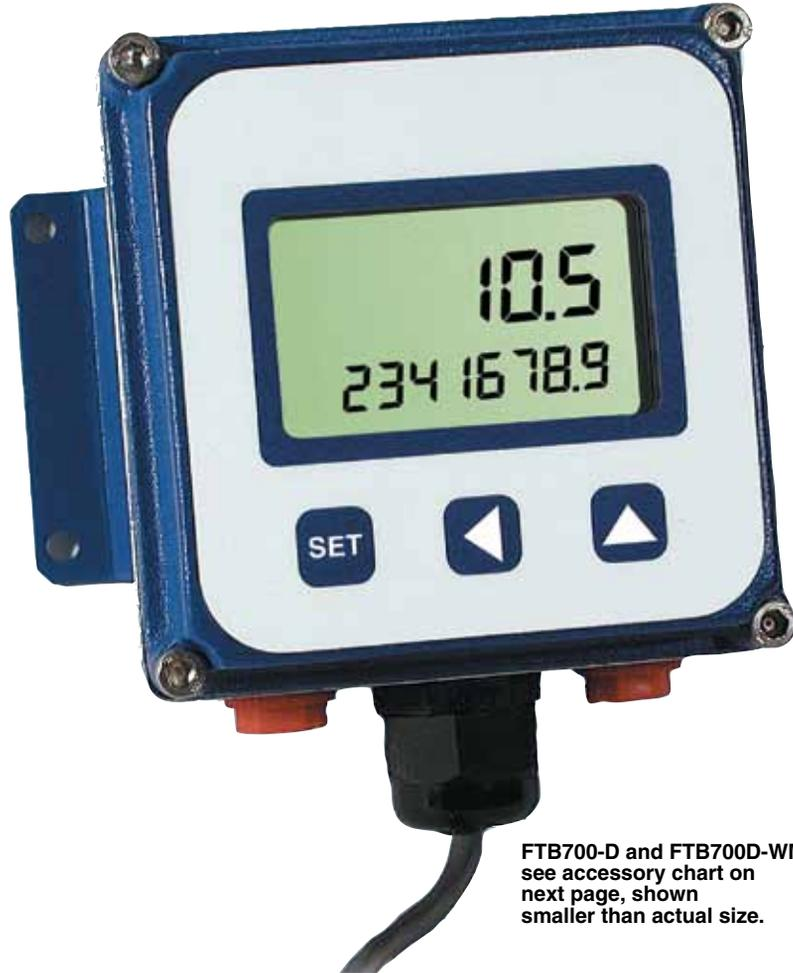
The FTB700-D Series flow displays are microcontroller-based indicator/transmitters that display flow rate and total and provide output signals. The FTB700-D is powered by external DC voltage and has both pulse and 4 to 20 mA analog outputs. When the FTB700-D is being used in the 4 to 20 mA mode, it is a "two-wire" or "loop-powered" device, meaning that the 4 to 20 mA output signal doubles as its power supply.
