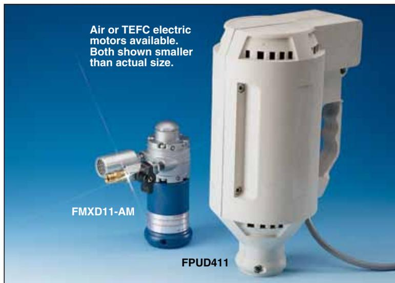
The air-driven 3/4 HP motor operates with 10 to 15 CFM air at 3.4 to 6.2 bar (50 to 90 psig), and includes a flow regulator and muffler.
