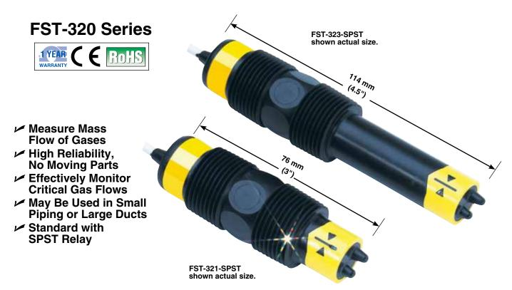
OMEGA's FST-320 Series thermal dispersion flow switches, especially designed for use with gases, sense changes in the heat transfer characteristics of the gases. Flow velocities from 1 to 90 fps are effectively monitored. The flow switch incorporates a standard SPST Relay switch output for control flexibility. OMEGA® controllers can easily be interfaced to perform a variety of control functions. The FST-320 family of sensors can be easily installed in line sizes ranging from ¾ to 12".
