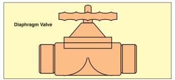
Diaphragm valves feature an abrasion-resistant and non-clogging design, with no small flow passages. They are good for many slurries and ultra-pure applications. The valve closes bubble-tight, and has a top-entry design for simple in-line maintenance. Suitable for on/off and throttling applications. Position indicator is included as standard. PVC valve body available with choice of EPDM or PTFE diaphragm.
