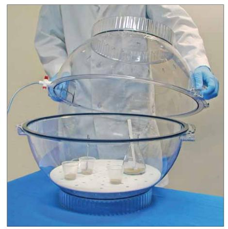
This large, domed desiccator is made from laboratory grade polycarbonate for a clear, unobstructed view of contents. Users will appreciate the roomy interior, portability and ease of use. Gas-port accepts ¼" I.D. tubing and has an easy turning PTFE stopcock which allows for the gentle entrance of air and minimal disturbance to the inside chamber and its contents.
