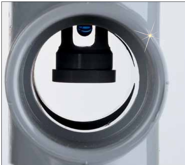
End cap seal and electrode, shown within pipe line. A quarter turn, and a pull seals the electrode assembly from line pressure.
