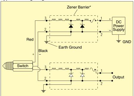
\* Source voltage not greater than 250 Vac. Zener barriers must be installed in accordance with barrier manufacturer's instructions.
