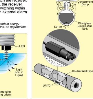
**Note:** The **LV170** sensor is a non-voltage-producing device and does not contain energy storing components. However, because primary use is in hazardous locations, an appropriate intrinsically safe interface device is required for its use.
