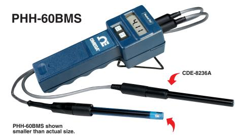
Detachable electrode, PHE-8200B on 1 m (3') extension cables, PHE-8236B.
