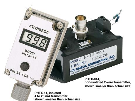
The model PHTX-014 pH two wire transmitter is designed to provide a standard 4 to 20 mA current output which is proportional to the pH being measured. Its small size and encapsulated construction allow for easy installation and will accommodate any pH electrode with a BNC connector. Temperature compensation is either manual or automatic with use of any  $1000\Omega$  Platinum RTD.
