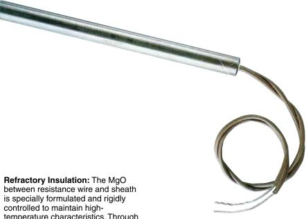
temperature characteristics. Through special processes it is densely compacted to improve its thermal conductivity and dielectric strength.
