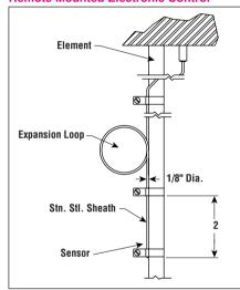
High Limit Controls — Electronic high limit controls can be mounted on the heater chamber with an overheat thermocouple welded to heating element sheath inside the chamber. This arrangement provides protection by shutting down the heater at a predetermined element sheath temperature. Option also available with thermocouple only, welded or clamped to heater element sheath as shown above.
