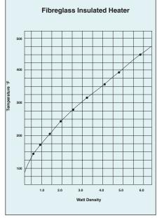
The temperature shown is the internal metallic element temperature. This would be the hottest point of the heater. The test heater was suspended horizontally in still air at a 70°F ambient temperature.
