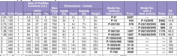
Ordering Example: P-25/120/3SH, 120 Vac power, 1 phase, 0.5 kW melt pot with 3-heat switch, \$686.
