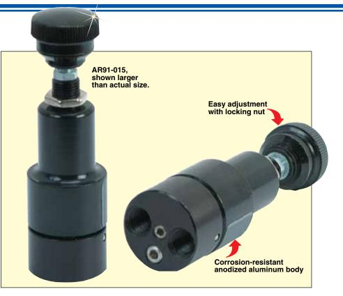
The AR91 and AR92 Series miniature pressure regulators are compact, low-cost units that operate in pressure ranges up to 100 psi, with a maximum supply pressure of 250 psi. They provide dependable reliability and accuracy for low-flow and dead-end applications, but are not designed for critical flow applications. Each unit has a corrosion-resistant anodized aluminum body with a standard fluorocarbon diaphragm.
