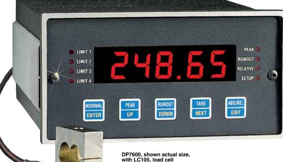
The text at the top of the switch (NORMAL, PEAK, RUNOUT, TARE, ABS/REL) indicates its normal function. The text at the lower half of the switch (ENTER, UP, DOWN, NEXT, EXIT) indicates the switch's function during setup and calibration.
