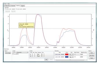
Charting Window – The charting window allows you to see your data graphed in real time. The Y axis is configurable to allow simultaneous graphing of multiple engineering units. You can output the image of your data to a .png file.
