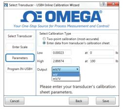
Field Calibration – The IN-USBH can easily be field calibrated with your mV transducer using OMEGA's free software wizard, utilizing known weights or pressures, or the transducer's calibration sheet. See the IN-USBH Quickstart guide for instructions on field calibration.
