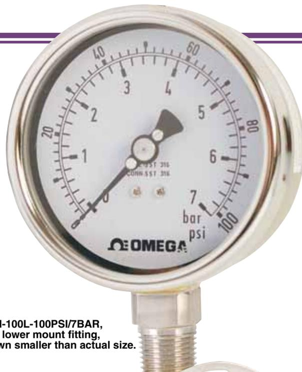
PGM-100L-100PSI/7BAR, with lower mount fitting, shown smaller than actual size.
