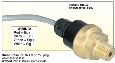
Wetted Parts: Brass, borosilicate, silicon, RTV and epoxy Vibration: 10 g, 55 to 2000 Hz Shock: 30 g Process Connection: ½ NPT male Electrical Connection: 0.4 m (18") 24-gage shielded cable Weight: 142 g (5 oz) Dimensions: 1½ hex; 72 H x 29.7 mm Dia. (2.84 x 1.17")
