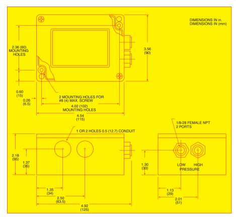
Overpressure: 2x operating static pressure (see To Order table) Pressure Connection: 1/2-28 female
