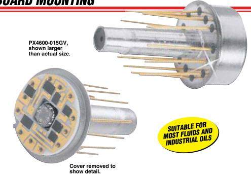
and span to tight tolerances. The unusually high performance of this transducer comes from a 4-active-arm bridge sensor using a micromachined diffused silicon diaphragm and proprietary thin-film media and dielectric isolation barriers. See next page for specifications.
