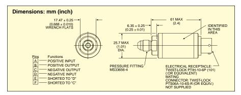
Reliability: MTBF = 100,000 hours Operating Temp Range: -54 to 150°C (-65 to 300°F) Compensated Temp Range:
